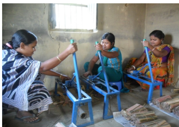
Artisans using Slicing machine to make slices out of the bamboo cylinders
