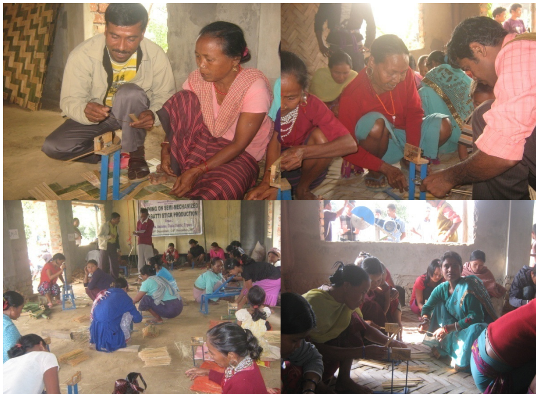
Artisans producing bamboo sticks with the semi mechanized stick making tools under the guidance of resource person during the training
